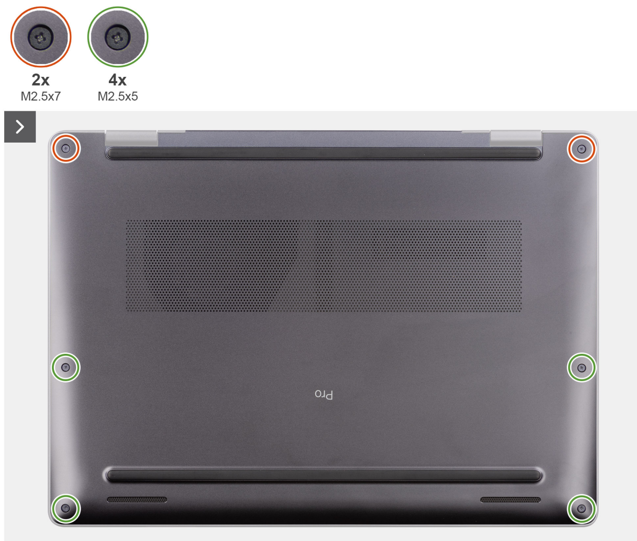
Rysunek 4. Removing the base cover
