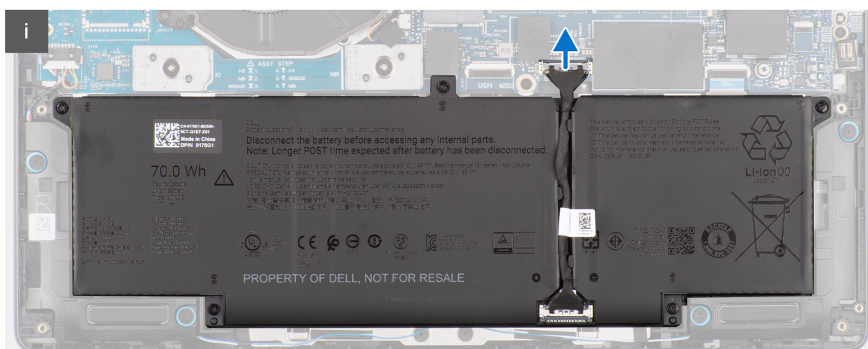
Rysunek 6. Disconnecting the battery cable
