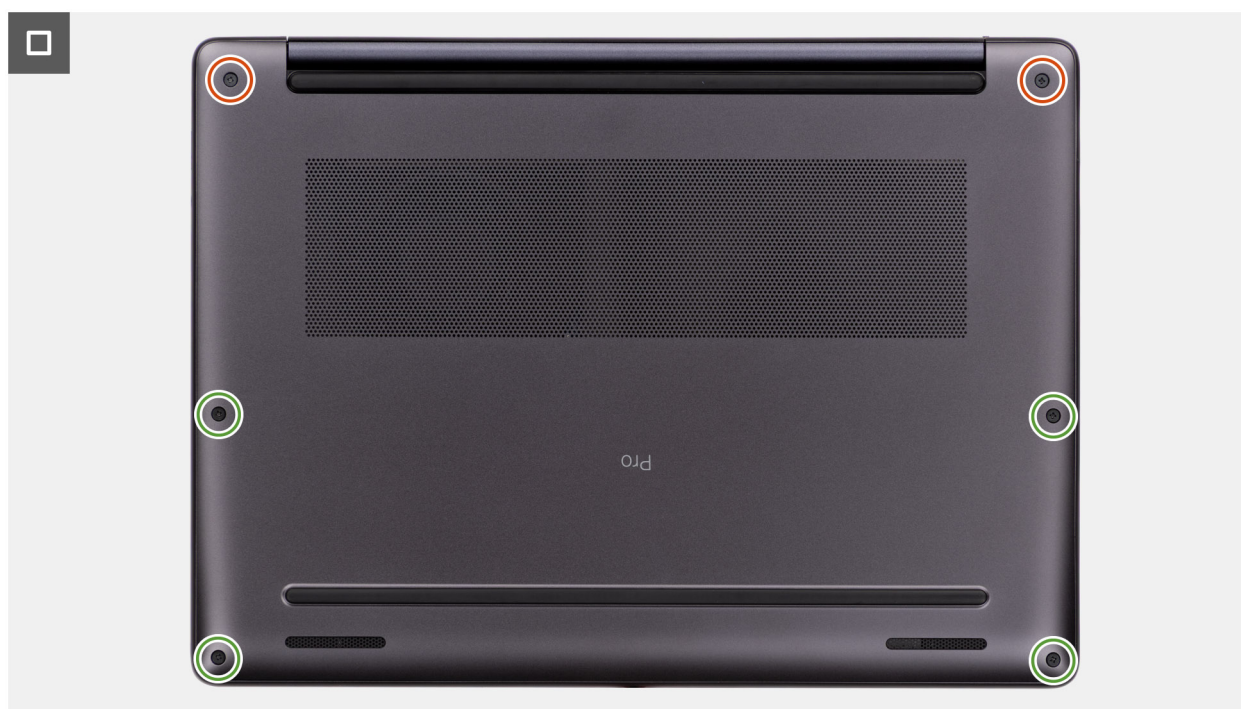
Rysunek 9. Installing the base cover
