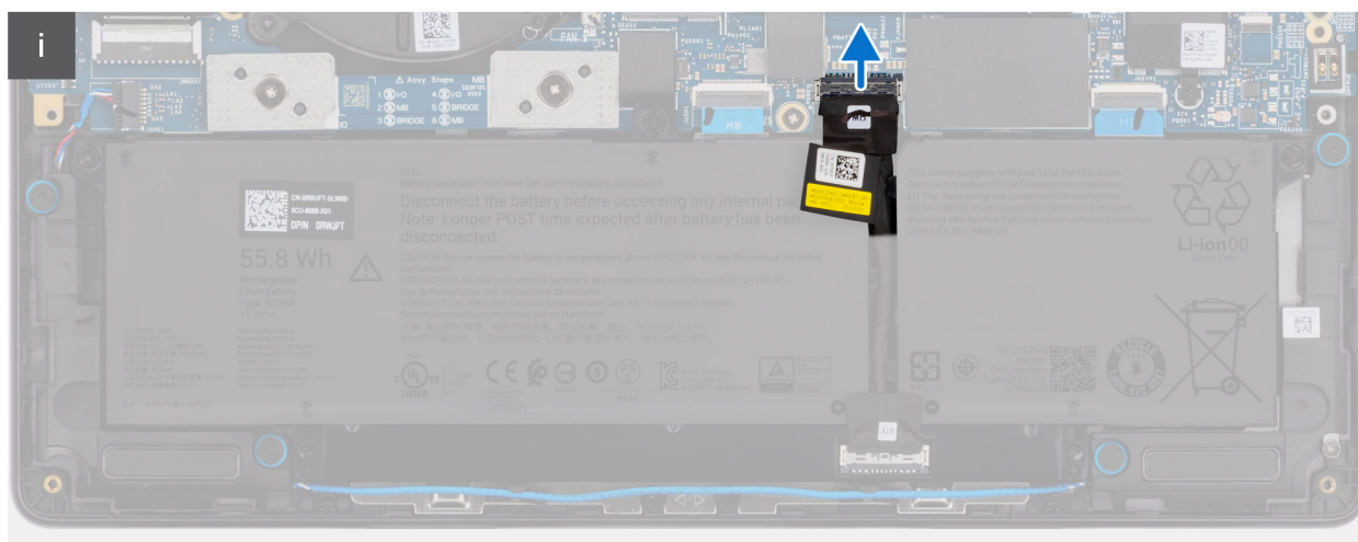
Rysunek 6. Disconnecting the battery cable
