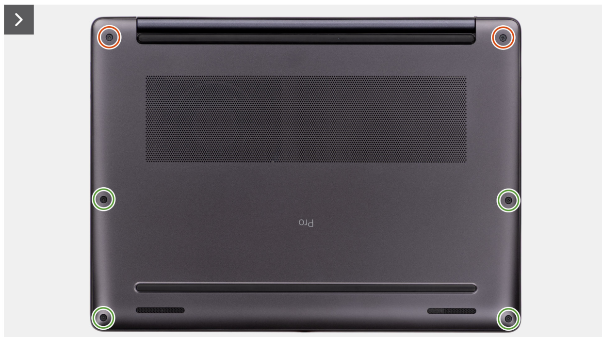
Rysunek 4. Removing the base cover
