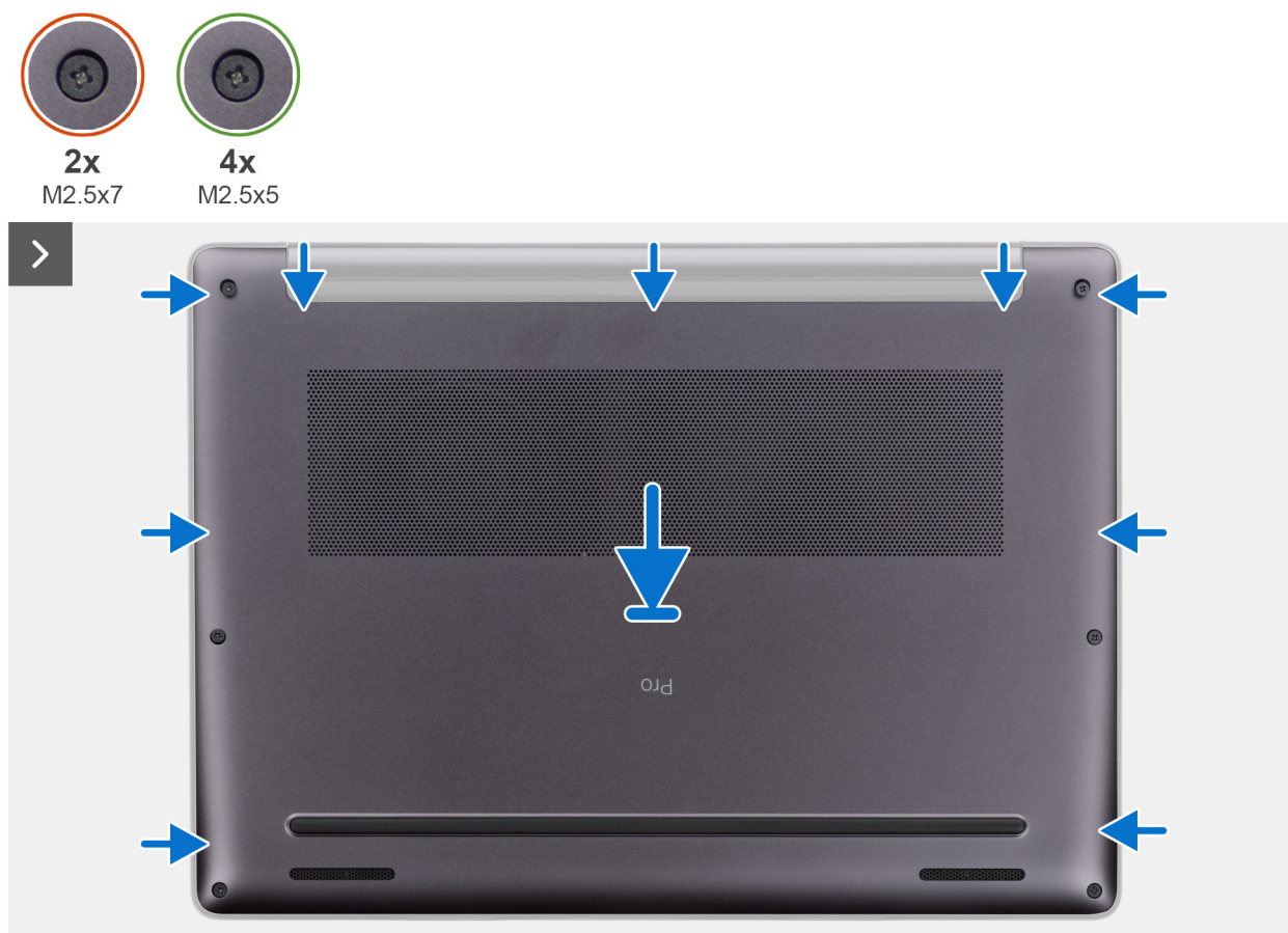
Rysunek 8. Installing the base cover
