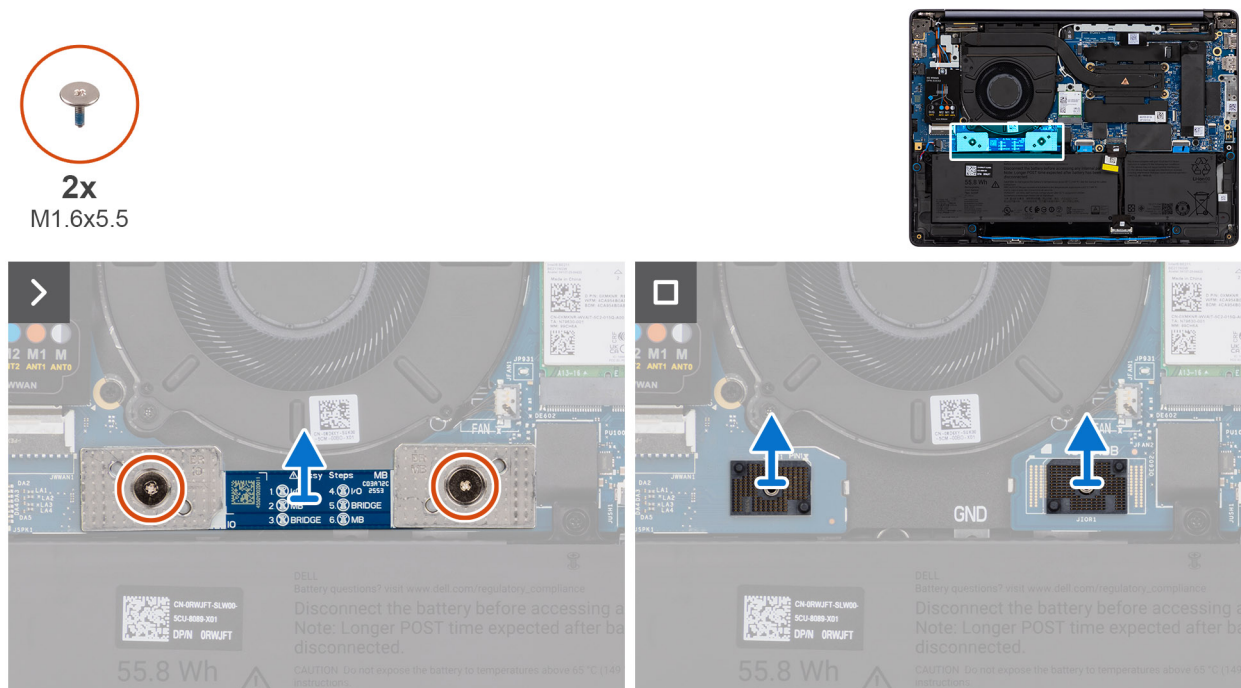
Rysunek 38. Removing the I/O-bridge board
