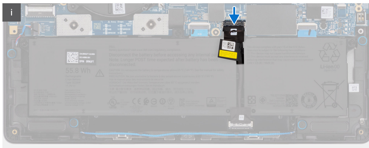
Rysunek 7. Connecting the battery cable
