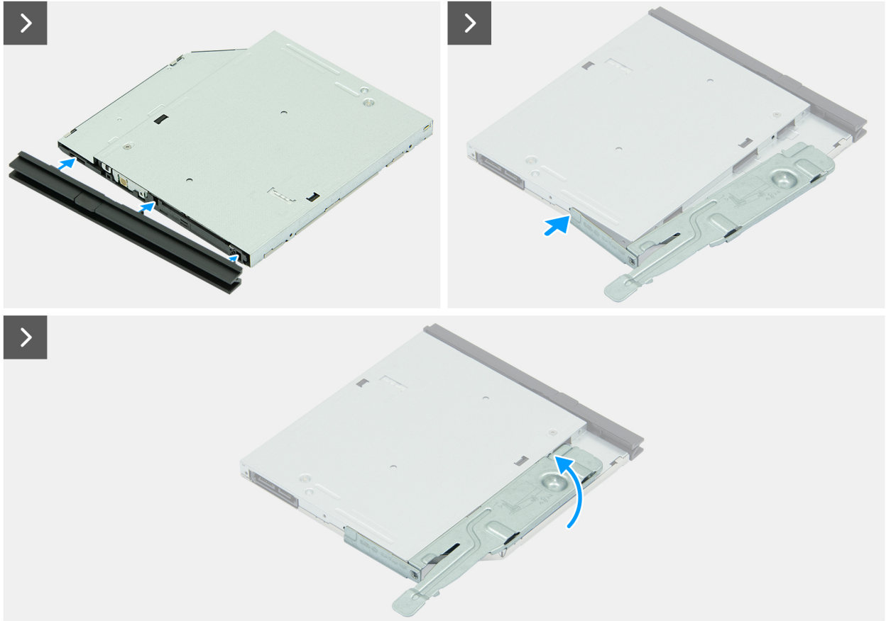
Rysunek 33. Installing the optical drive
