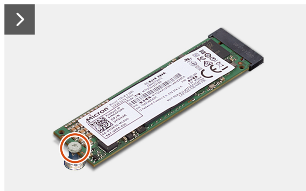
Rysunek 24. Removing the M.2 2280 solid state drive
