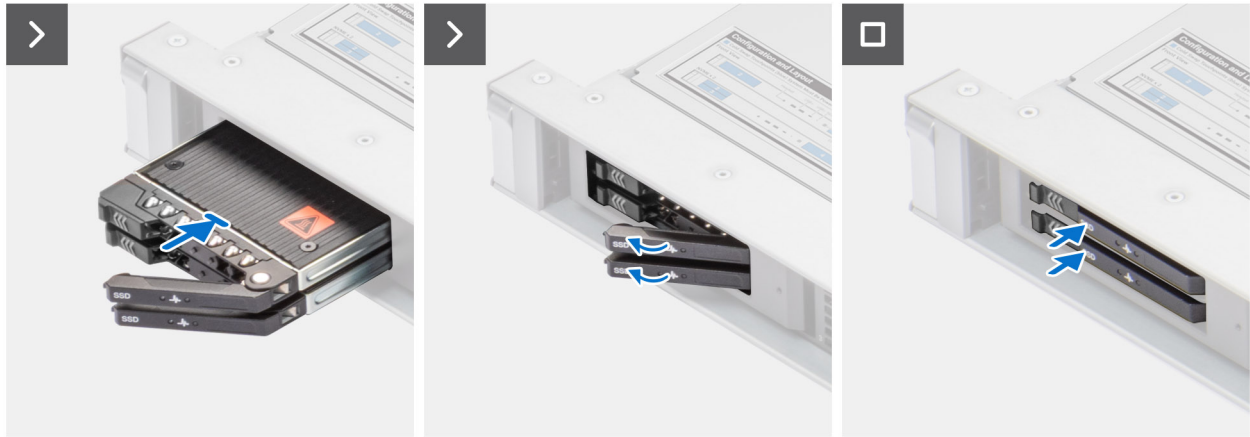
Figure 7. Installing the front M.2 NVMe SSD carrier and tray
