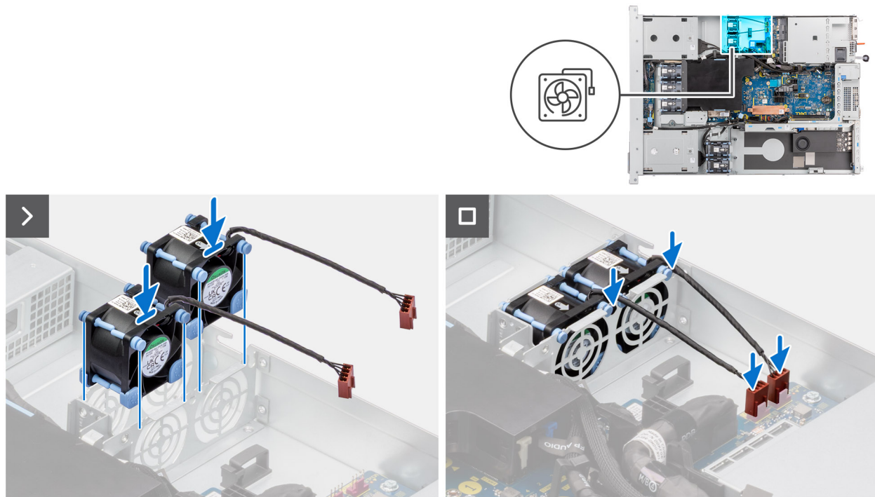
Figure 31. Installing the PSU fans
