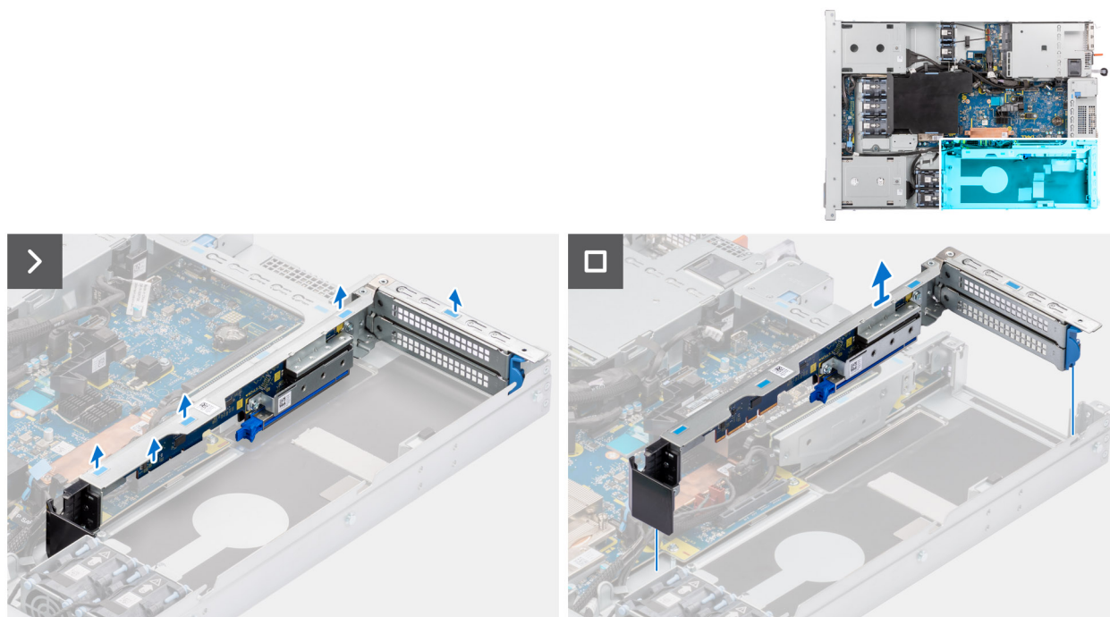
Figure 44. Removing the riser1 module
