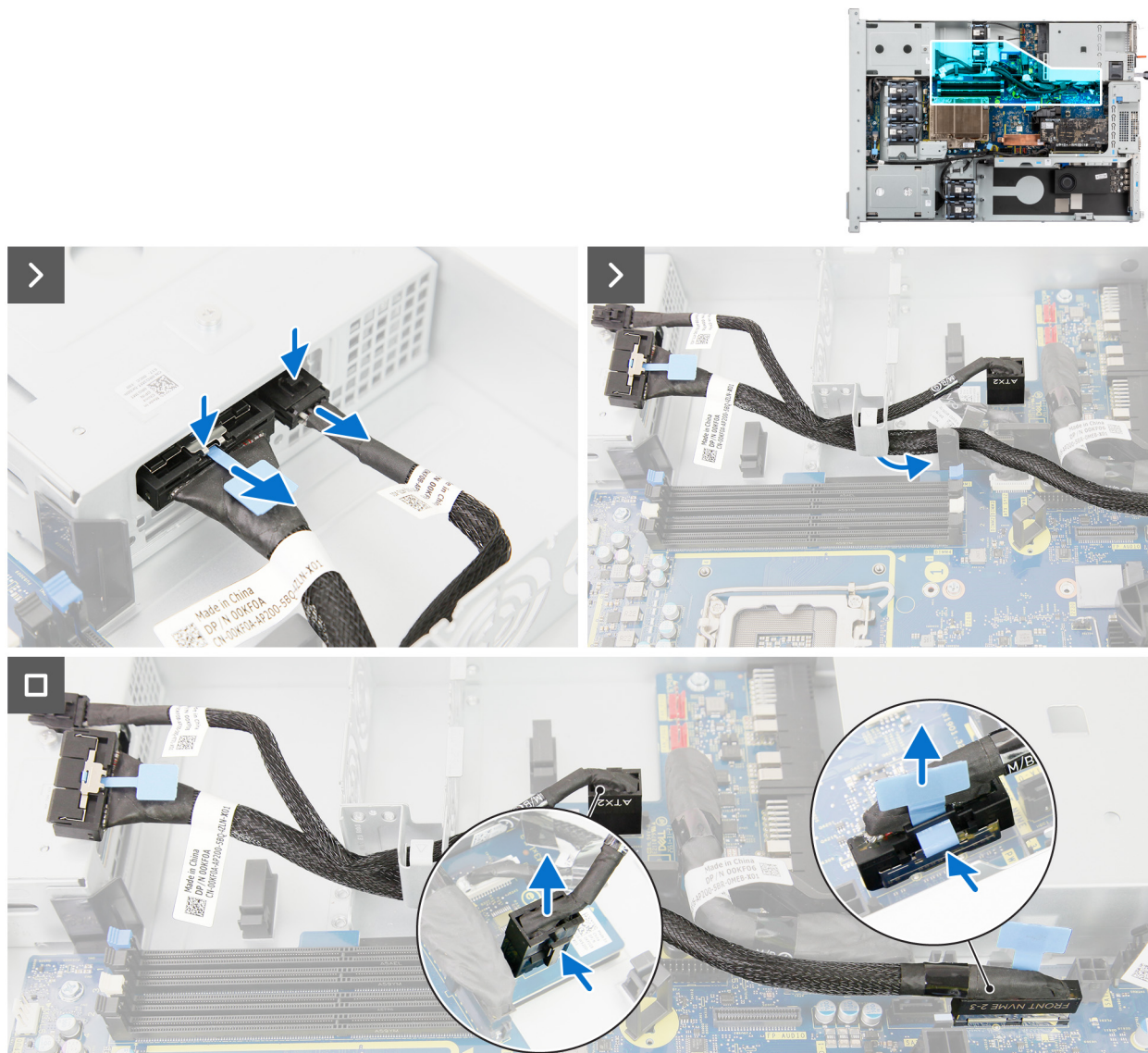
Figure 58. Removing the NVMe SSD cables
