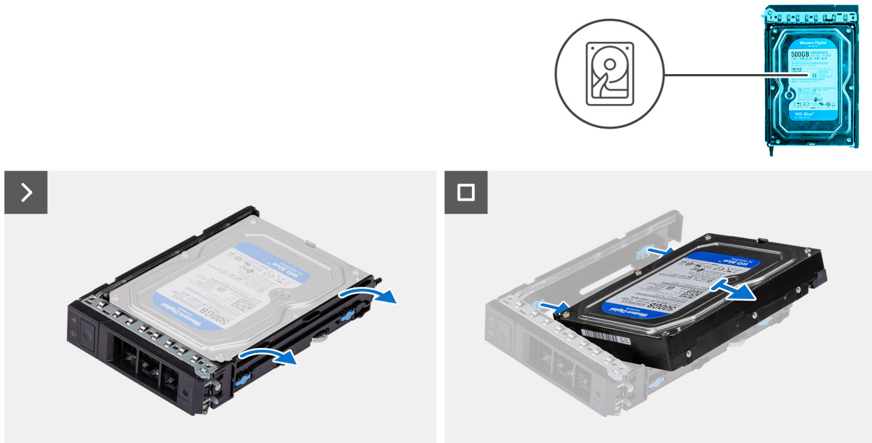
Figure 15. Removing the external hard-drive carrier
