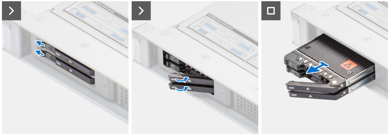
Figure 6. Removing the front M.2 NVMe SSD carrier and tray
