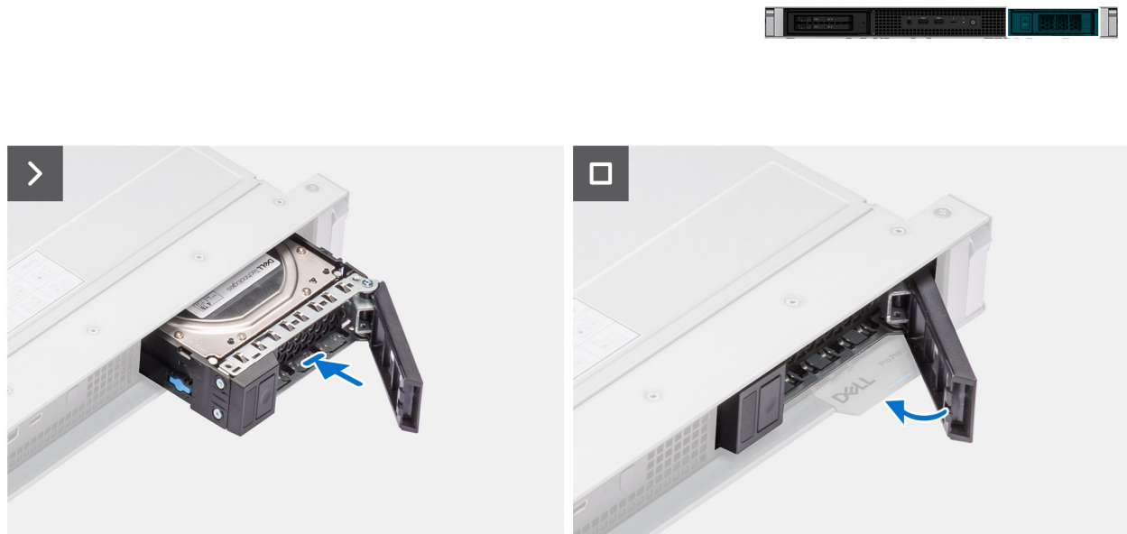
Figure 14. Installing the external hard-drive assembly
