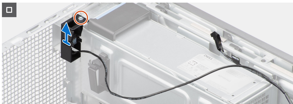
Figure 67. Removing the intrusion switch
