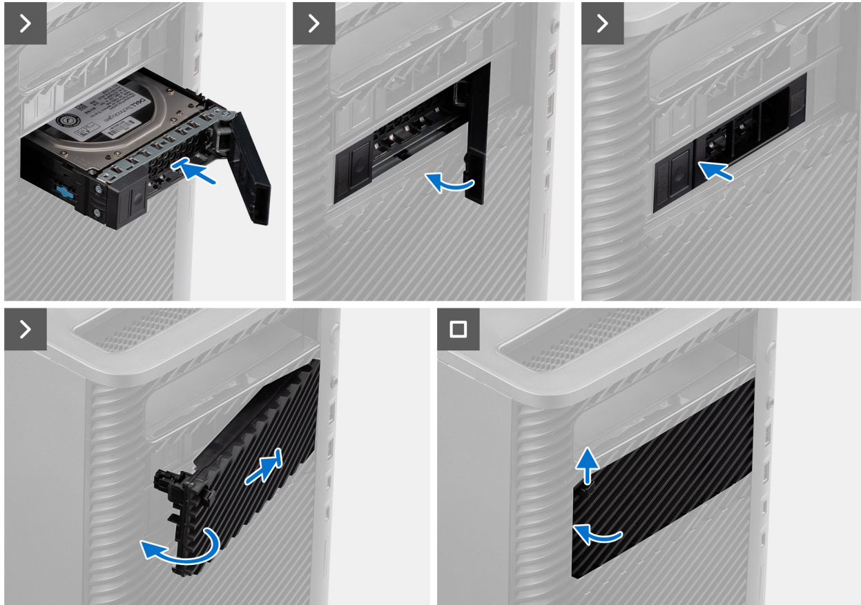
Figure 46. Installing the external hard drive assembly
