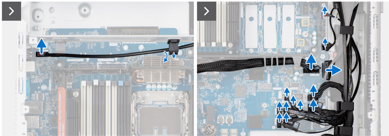
Figure 105. Removing the system board
