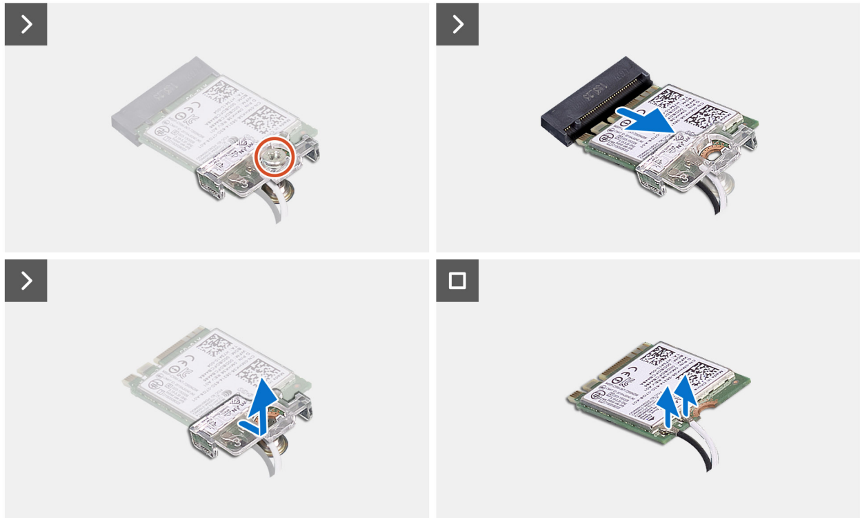
Figure 62. Removing the wireless card
