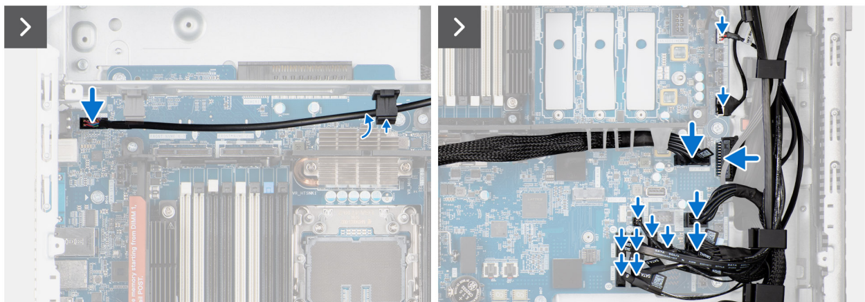
Figure 110. Installing the system board
