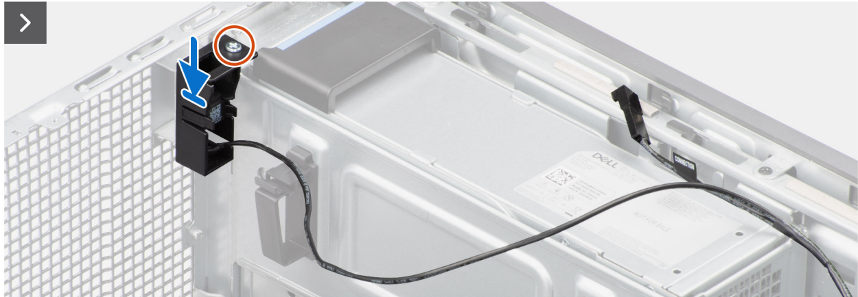
Figure 68. Installing the intrusion switch
