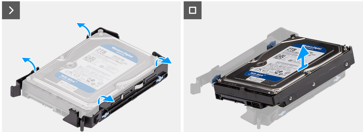
Figure 55. Removing the 3.5-inch hard drive bracket
