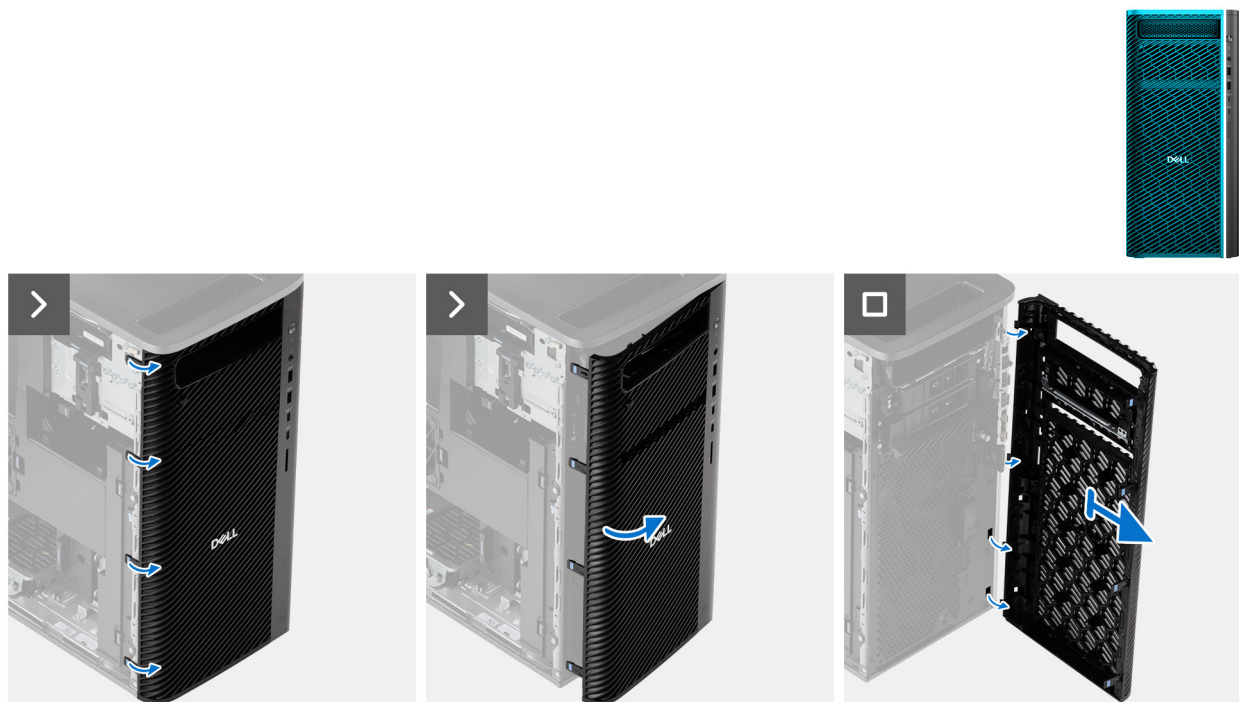
Figure 27. Removing the front bezel
