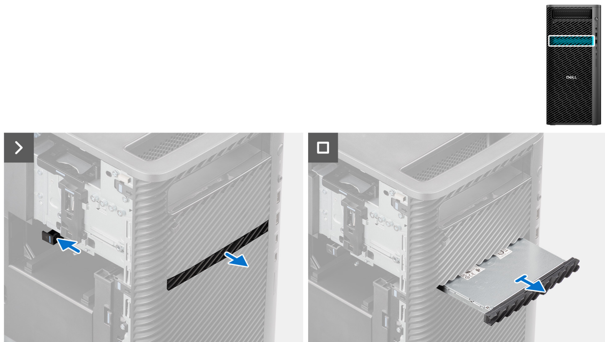
Figure 39. Removing the optical drive
