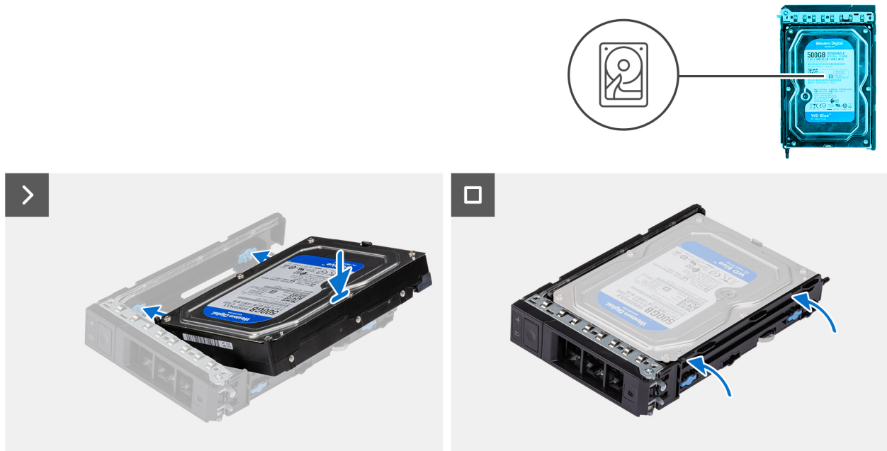
Figure 33. Installing the external hard-drive carrier
