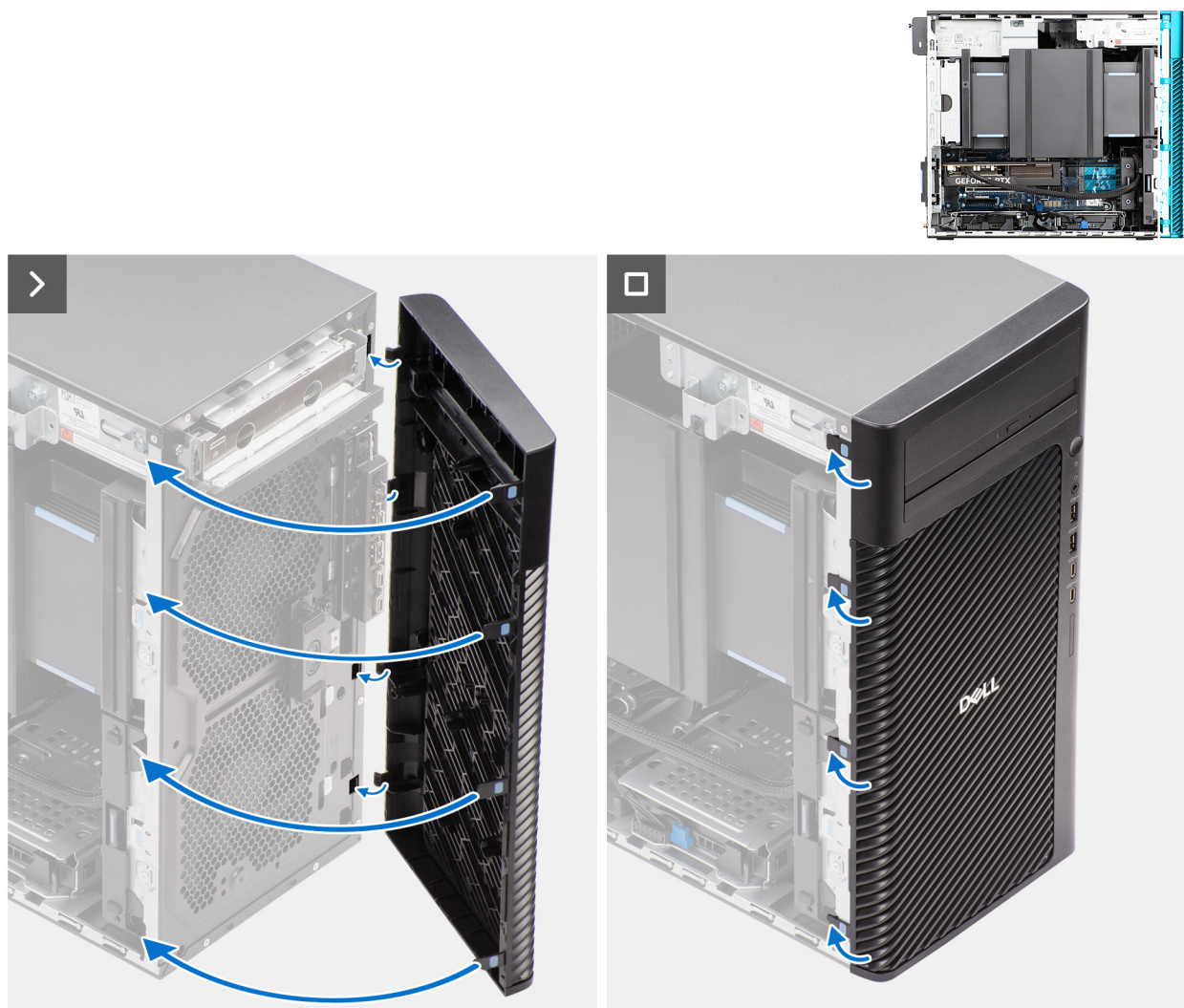
Figure 22. Installing the front bezel
