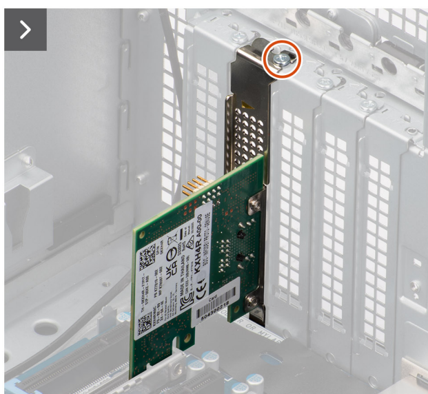
Figure 82. Installing the Intel Ethernet Controller I226-V
