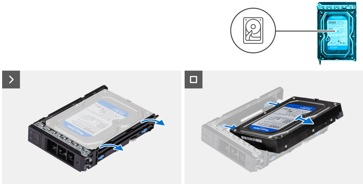
Figure 32. Removing the external hard-drive carrier
