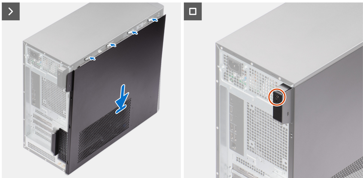
Figure 18. Installing the side cover
