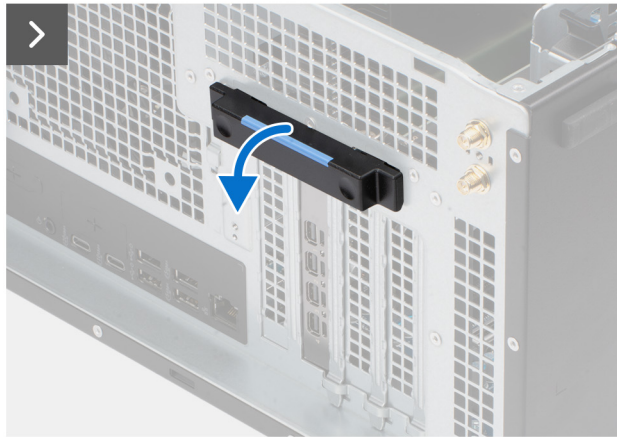
Figure 67. Removing the nonpowered graphics card
