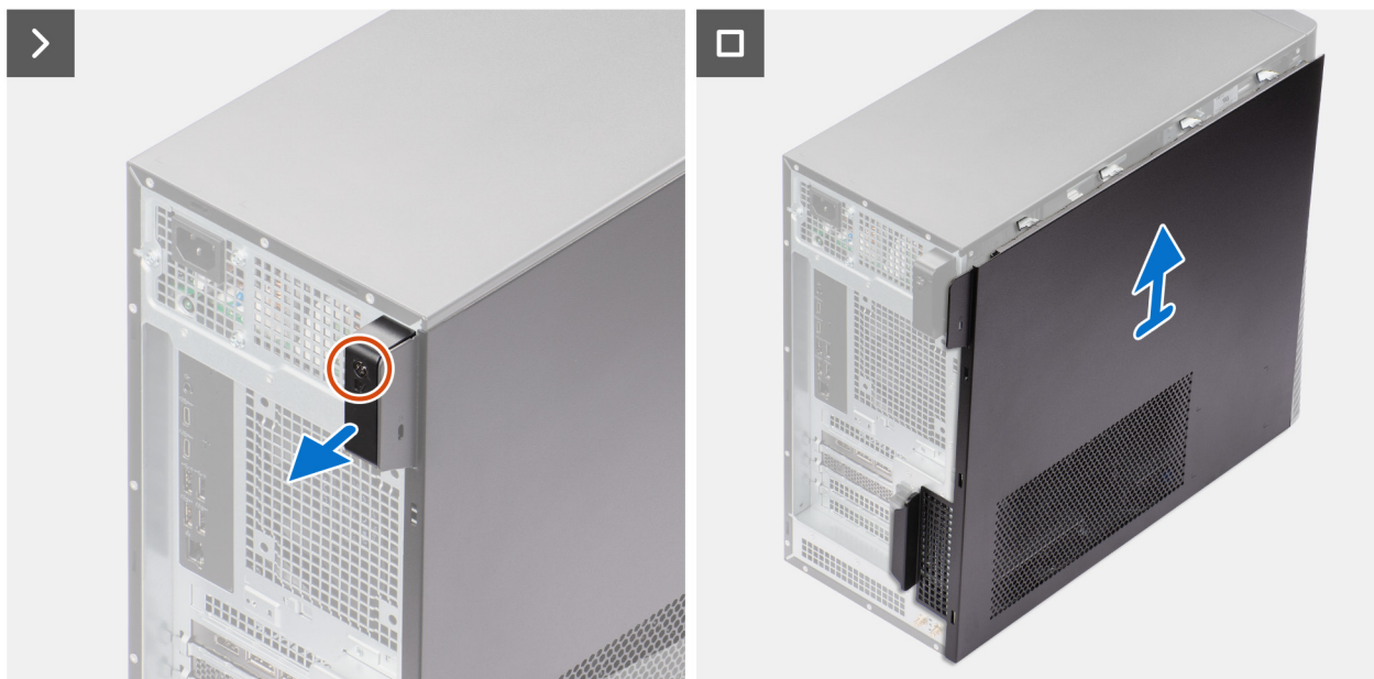
Figure 17. Removing the side cover
