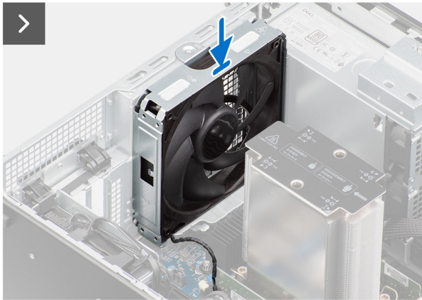
Figure 62. Installing the rear chassis fan
