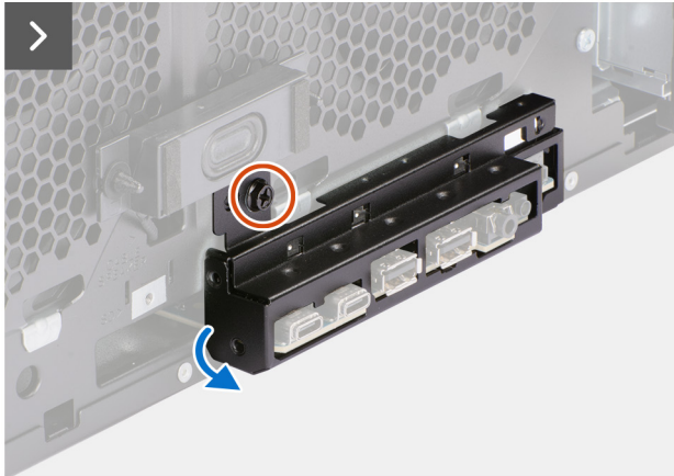
Figure 23. Removing the front I/O-bracket
