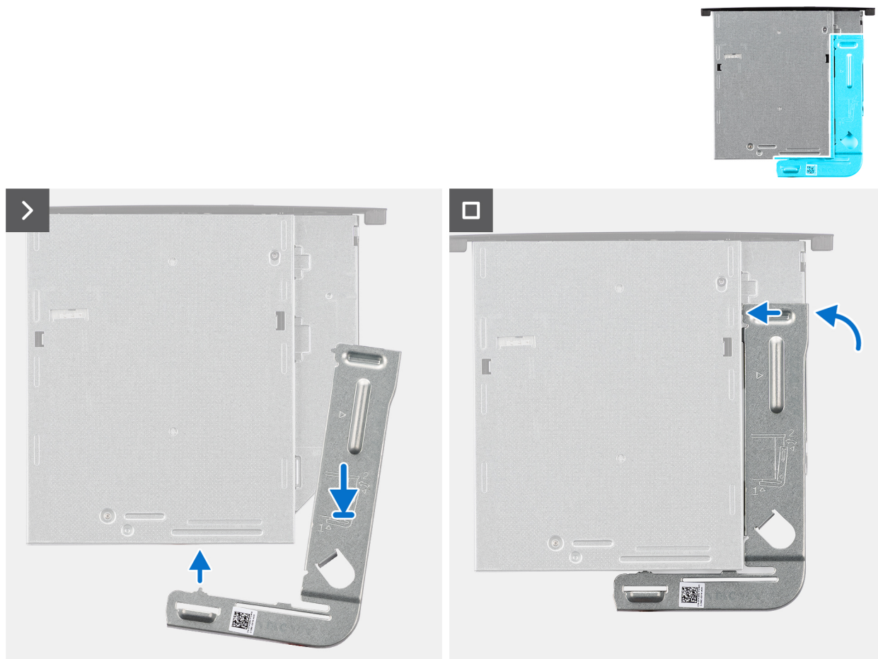
Figure 28. Installing the optical-drive bracket
