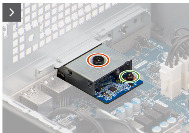
Figure 111. Installing the optional dual-USB 3.2 module
