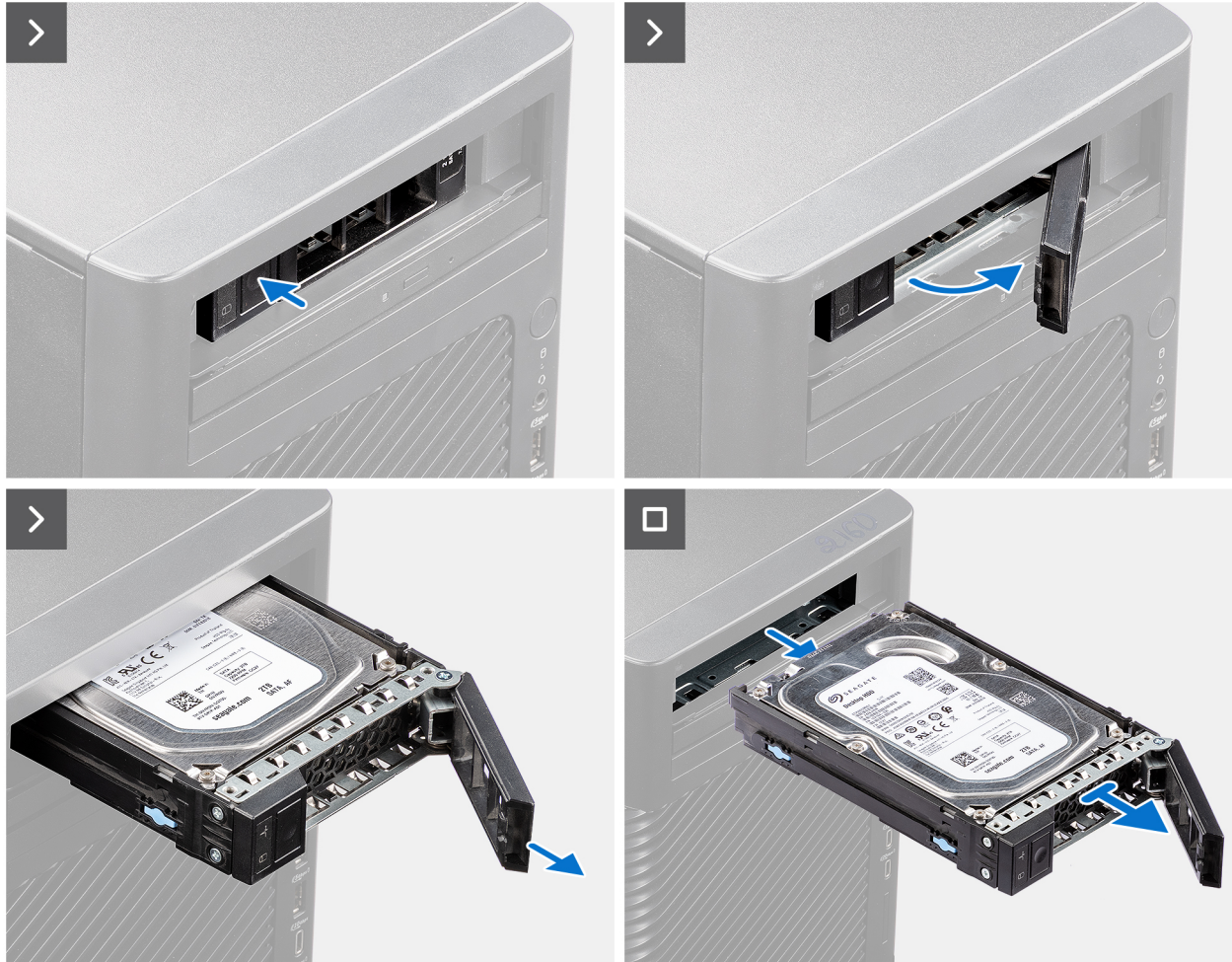
Figure 31. Removing the external hard-drive assembly
