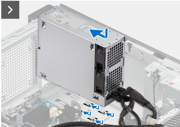
Figure 89. Installing the PSU
