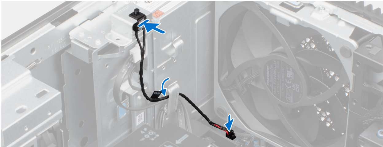
Figure 56. Installing the intrusion switch
