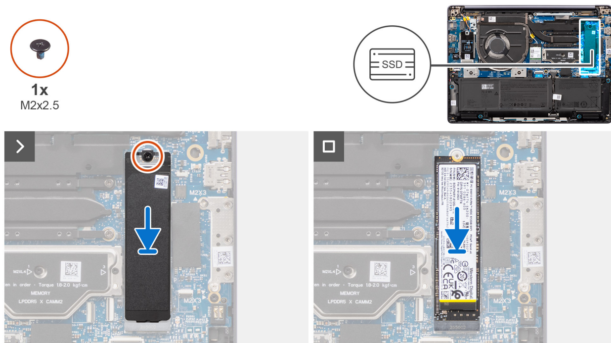
Rysunek 18. Installing the 2280 solid-state drive (LPCAMM2 memory)
