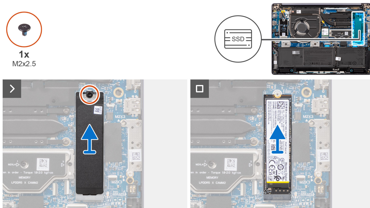
Rysunek 17. Removing the 2280 solid-state drive (LPCAMM2 memory)
