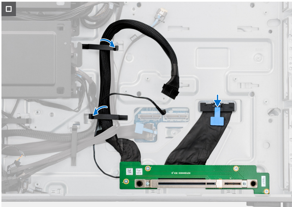
Figure 137. Installing the HEPCB board
