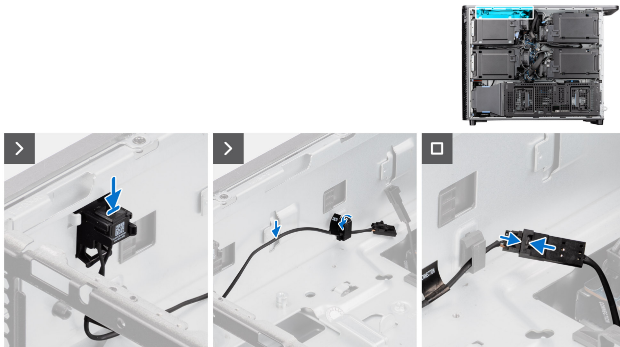
Figure 97. Installing the expansion intrusion switch
