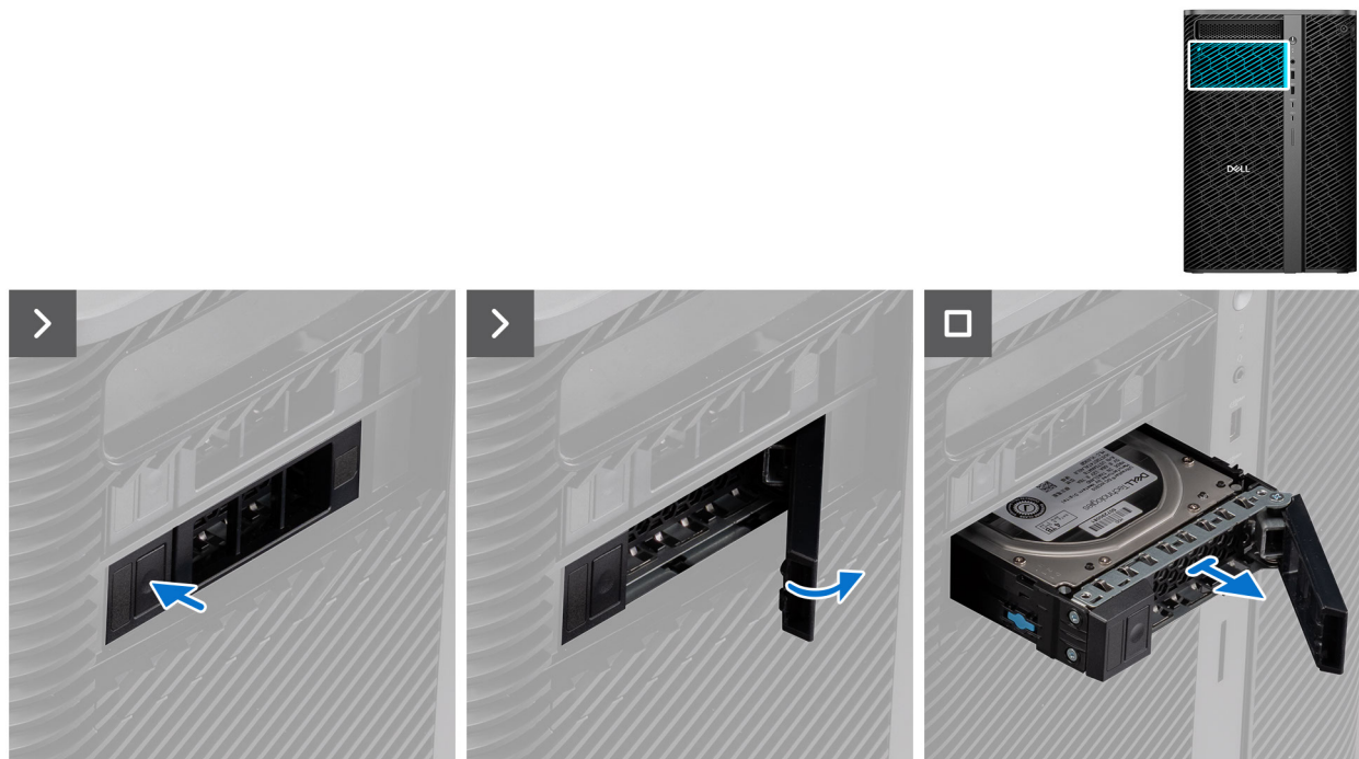
Figure 62. Removing the external hard drive assembly
