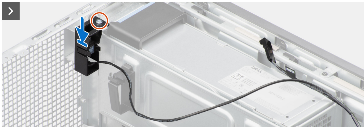
Figure 94. Installing the base intrusion switch
