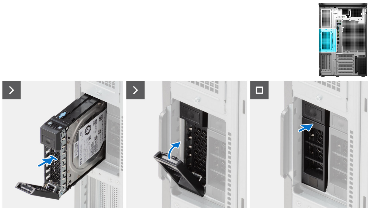
Figure 72. Installing the external rear hard drive assembly
