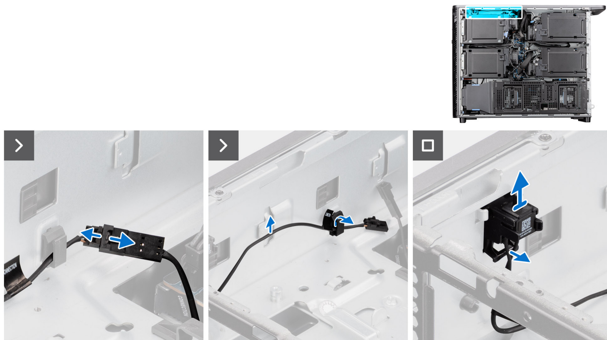
Figure 96. Removing the expansion intrusion switch
