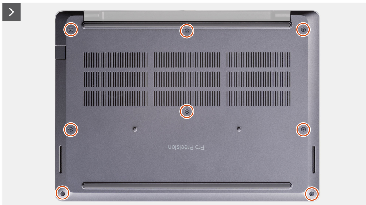
Rysunek 2. Loosen the captive screws
