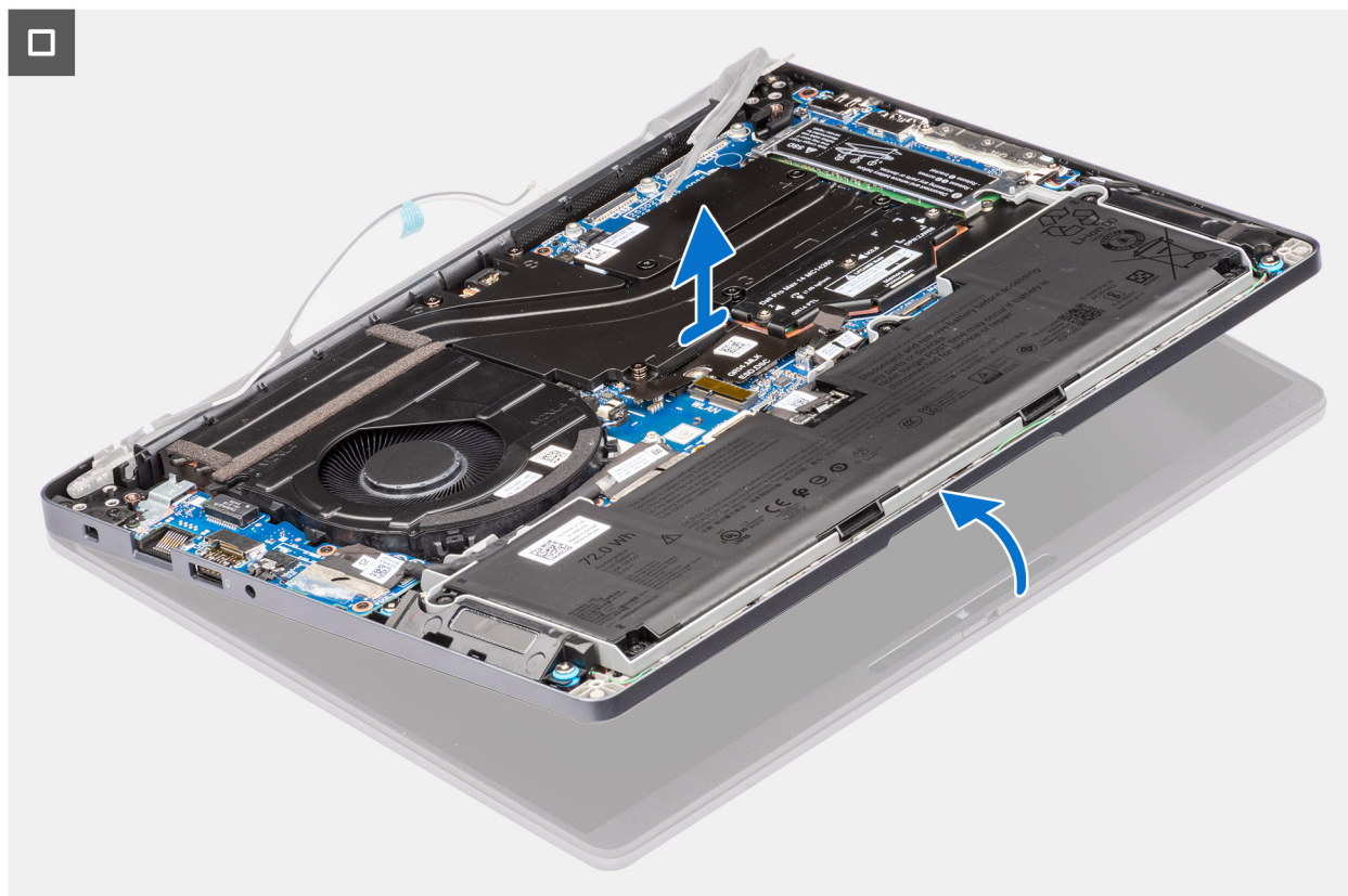
Rysunek 38. Removing the display assembly
