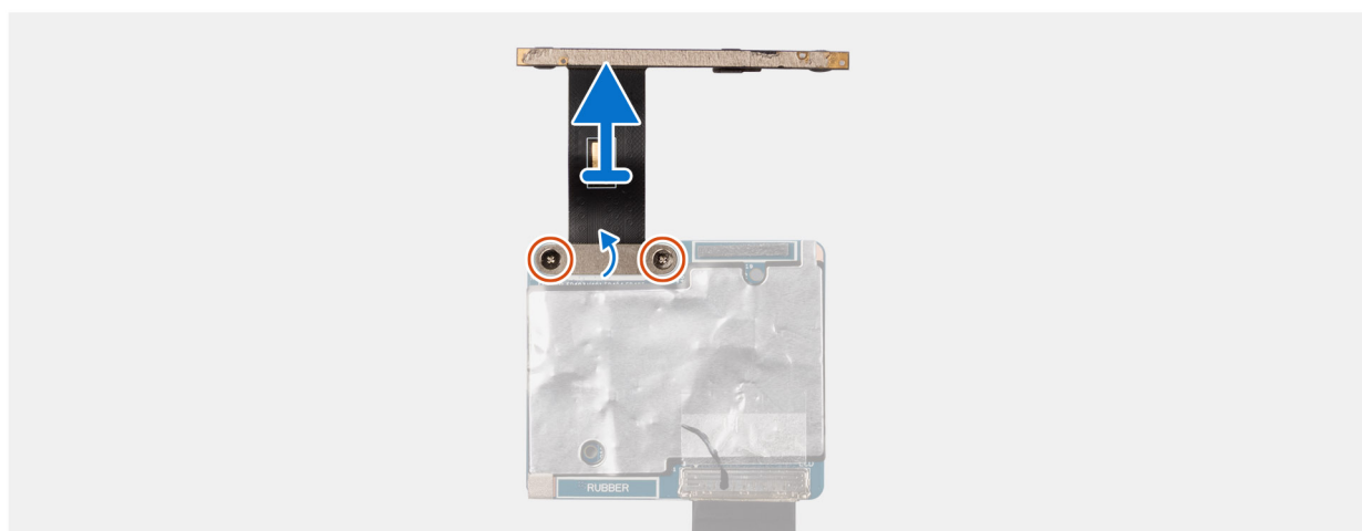
Rysunek 61. Removing the camera
