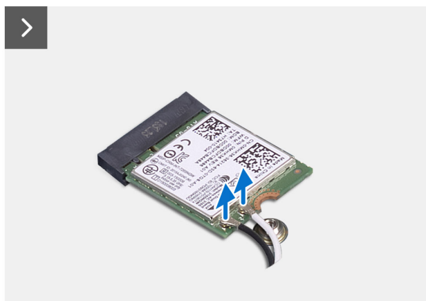
Rysunek 16. Removing the wireless card
