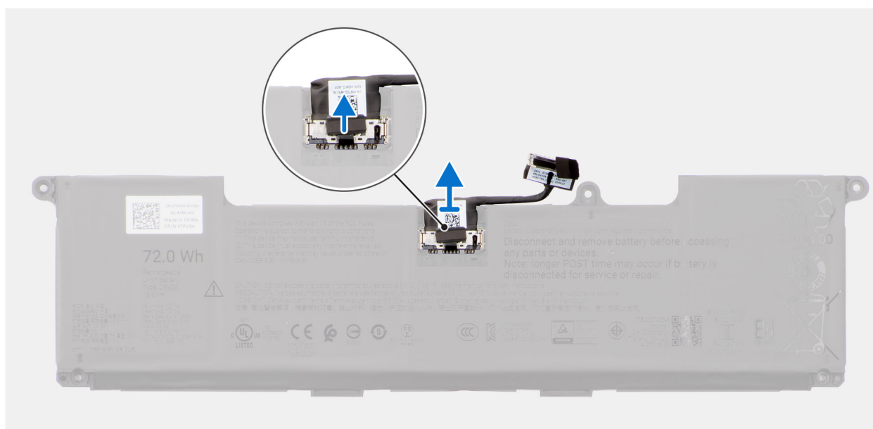
Rysunek 8. Removing the battery cable
